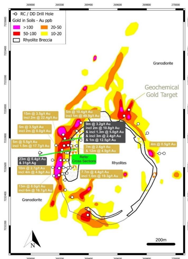
Figure 3: Red Mountain Breccia Pipe Target Showing Gold Soil Anomalies and Drill Collar Locations with Planned DD Holes
