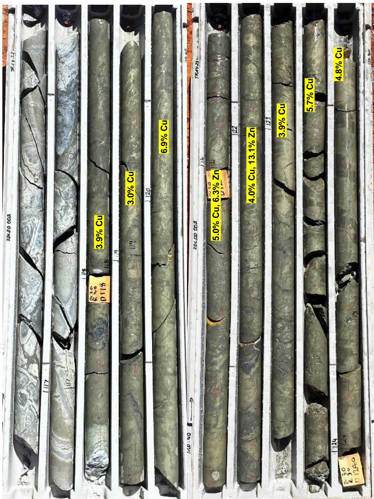
Figure 1: Develin Creek –New Zenith Diamond Drill Hole ZDCDD002 Example of Results Showing Consistent High-grade Copper values (116m – 124.8m) – refer ASX Release 5-Jul-21 for further details).
